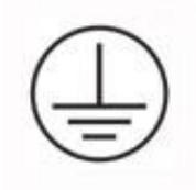
Grounding work should be made for safety and prevention of static electricity and noise failure. In addition, a ground wire should be installed independently without sharing the wire with other products. At grounding work, please be sure to contact our distributor near you or our designated dealers. In case of electrical leakage when grounding is insufficient or not connected, it may cause fire and/or electric shock.
