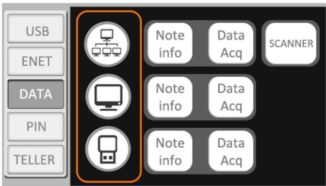
By Network, USB Cable and USB Stick, Note Information, Data Acquisition and Scanned data are transferred
